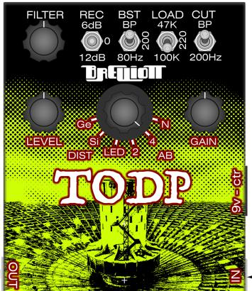
GAIN: continuous gain, as used on classic 70s and 80s distortion pedals. Options: pedals come in Mid Range, Transparent OverDrive, Red Rocket, & Original Bass Version. The OBV does not have a "bright" cap, whereas all the others do.
